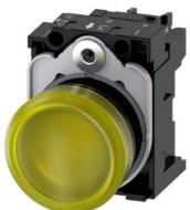
Indicator light, 22 mm, round, plastic, yellow, lens, smooth, with holder, LED module, with integrated LED 24 V AC/DC, screw terminal, with laser labeling, upper case and lower case, always upper case at beginning of line
