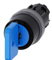
Key-operated switch O.M.R, 22 mm, round, plastic with metal front ring, lock number 73038, blue, with 2 keys, 3 switch positions I-O<II, left latching, right momentary contact type, actuating angle 2x45°, 10:30h/12h/13:30h, key removal O, with laser labeling, upper case
