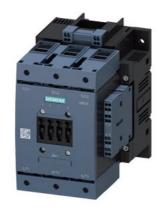
power contactor, AC-3 115 A, 55 kW / 400 V AC (50-60 Hz) / DC operation 200-220 V AC/DC auxiliary contacts 2 NO + 2 NC 3-pole, frame size S6 with box terminals drive: conventional spring-loaded terminal
