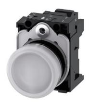
Indicator lights, 22 mm, round, plastic, white, lens, smooth, with holder, LED module, with integrated LED 230 V AC, spring-type terminal, with laser labeling, symbol number according to, ISO 7000 or IEC 60417
