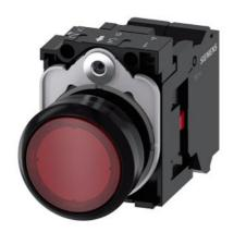
Illuminated pushbutton, 22 mm, round, plastic, red, pushbutton, flat, momentary contact type, with holder, 1NC, LED module with integrated LED 24 V AC/DC, spring-type terminal, with laser labeling, upper case and lower case, always upper case at beginning of line
