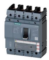
circuit breaker 3VA5 UL frame 250 breaking capacity class C 100kA @ 480V 4-pole, line protection TM230, FTAM, In=200A overload protection Ir=200A fixed short-circuit protection Ii=5...10 x In N conductor unprotected without connection
