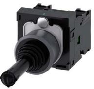
Coordinate switch, 22 mm, round, plastic with metal front ring, black, 2 switch positions, horizontal latching, without mechanical interlocking, in O position, with holder, 1 NO, 1 NO, screw terminal, with laser labeling, upper case
