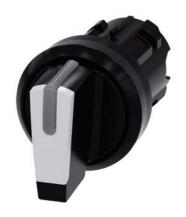
Selector switch, illuminable, 22 mm, round, plastic, white, selector switch, short, 3 switch positions I-O<II, left latching, right momentary contact type, actuating angle 2x45°, 10:30h/12h/13:30h, with laser labeling, inscription or symbol Customer-specific selection with SIRIUS ACT configurator (CIN)
