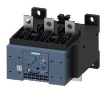
Overload relay 50...200 A for motor protection Size S6, CLASS 5...30E Contactor mounting/stand-alone installation Main circuit: busbar connection Auxiliary circuit: Spring-type terminal Manual-Automatic-Reset Internal ground fault detection
