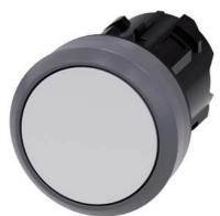
Pushbutton, 22 mm, round, plastic with metal front ring, white, pushbutton, flat momentary contact type, with laser labeling, symbol number according to, ISO 7000 or IEC 60417
