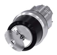
RONIS key-operated switch, 22 mm, round, metal, shiny, special lock, with 2 keys, 2 switch positions O-I, latching, actuating angle 90°, 10:30h/13:30h, key removal O+I, possible special locks: SB31, 421, 455
