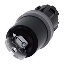
Key-operated switch IKON, 22 mm, round, plastic with metal front ring, lock number 360012K1, with 2 keys, 2 switch positions O-I, latching, actuating angle  $90^\circ, 10:30h/13:30h,$  key removal O, with laser labeling, upper case and lower case, always upper case at beginning of line
