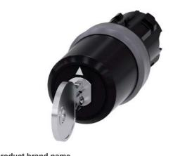
Key-operated switch BKS, 22 mm, round, plastic with metal front ring, lock number S1, with 2 keys, 3 switch positions I-O-II, latching, actuating angle 2x45°, 10:30h/12h/13:30h, Key removal I+O+II, with laser labeling, upper case and lower case, always upper case at the beginning of the word
