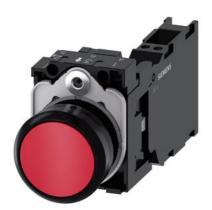
Pushbutton, 22 mm, round, plastic, red, pushbutton, flat, momentary contact type, with holder 1 NO+1 NC, spring-type terminal, with laser labeling, upper case
