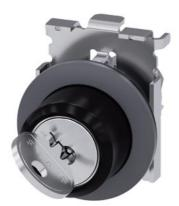
RONIS key-operated switch, 30 mm, round, Metal, matte, front ring for flush installation, lock number SB30, with 2 keys, 2 switch positions O-I, latching, actuating angle 90°, 10:30h/13:30h, key removal O+I, possible special locks: SB31, 421, 455, with laser labeling, lower case
