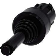
Coordinate switch, 22 mm, round, plastic, black, 4 switch positions, latching, with mechanical interlocking, with laser labeling, upper case and lower case, always upper case at the beginning of the word
