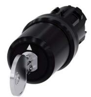
Key-operated switch BKS, 22 mm, round, plastic, lock number S1, with 2 keys, 3 switch positions I-O<II, left latching, right momentary contact type, actuating angle  $2x45^{\circ}$ , 10:30h/12h/13:30h, key removal I, with laser labeling, lower case
