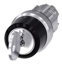
RONIS key-operated switch, 22 mm, round, metal, shiny, lock number SB30, with 2 keys, 3 switch positions I-O<II, left latching, right momentary contact type, actuating angle 2x45°, 10:30h/12h/13:30h, key removal I, possible special locks: SB31, 421, 455, with laser labeling, lower case
