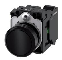
Pushbutton, 22 mm, round, plastic, black, pushbutton, flat, momentary contact type, with holder 1 NO, spring-type terminal, with laser labeling, inscription or symbol Customer-specific selection with SIRIUS ACT configurator (CIN)
