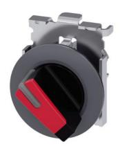
Selector switch, illuminable, 30 mm, round, Metal, matte, red, selector switch, short, front ring for flush installation, 2 switch positions O<I, momentary contact type, Actuating angle 45°, 10:30h/12h, with laser labeling, upper case
