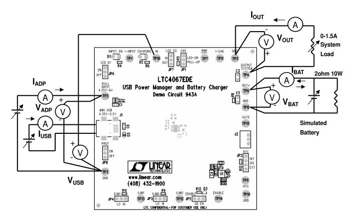
Figure 1. Proper Measurement Equipment Setup
