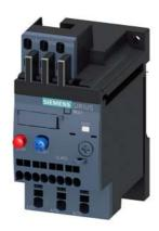
Overload relay 0.11...0.16 A Thermal For motor protection Size S00, Class 10 Stand-alone installation Main circuit: Spring-type terminal Auxiliary circuit: spring-type terminal Manual-Automatic-Reset
