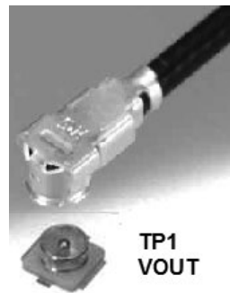
Figure 4. Technique for Measuring Output Ripple and Step Response with a Low Inductance Connector (Not Supplied)
