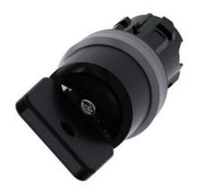
Key-operated switch O.M.R, 22 mm, round, plastic with metal front ring, lock number 73034, black, with 2 keys, 2 switch positions O<I, momentary contact type, Actuating angle 45°, 10:30h/12h, key removal O, with laser labeling, lower case
