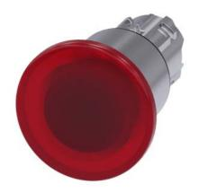
Illuminated mushroom pushbutton, 22 mm, round, metal, shiny, red, 40 mm, 3 switch positions, latches after pushing in, unlatches by pull-to-unlatch mechanism to center position, after pulling out the button Retraction to center position, with laser labeling, inscription or symbol Customer-specific selection with SIRIUS ACT configurator (CIN)
