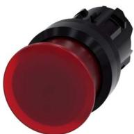
Illuminated mushroom pushbutton, 22 mm, round, plastic, red, 30 mm, momentary contact type, with laser labeling, upper case and lower case, always upper case at beginning of line
