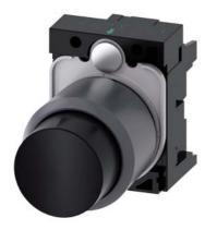
Pushbutton, compact, with extended stroke (12 mm), 22 mm, round, plastic with metal front ring, black, pushbutton, high, momentary contact type, with holder, with laser labeling, upper case
