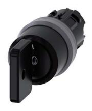
Key-operated switch O.M.R, 22 mm, round, plastic with metal front ring, lock number 73034, black, with 2 keys, 3 switch positions I-O<II, left latching, right momentary contact type, actuating angle 2x45°, 10:30h/12h/13:30h, key removal I, with laser labeling, upper case and lower case, always upper case at the beginning of the word
