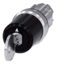
key-operated switch Siemens, 22 mm, round, metal, shiny, lock no. STGH10, with 2 keys, 3 switch positions I>O<II, momentary contact type, actuating angle 2x45°, 10:30h/12h/13:30h, key removal O, with laser labeling, inscription or symbol customer-specific selection with SIRIUS ACT configurator (CIN)
