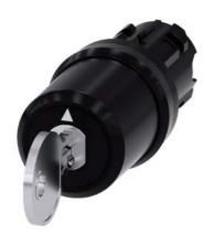
key-operated switch Siemens, 22 mm, round, plastic, lock number SSG10, with 2 keys, 3 switch positions I>O<II, momentary contact type, actuating angle 2x45°, 10:30h/12h/13:30h, key removal O, with laser labeling, upper case
