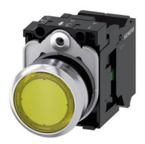
Illuminated pushbutton, 22 mm, round, metal, shiny, yellow, pushbutton, flat, momentary contact type, with holder, 1NO, LED module with integrated LED 110 V AC, spring-type terminal, Z=20-unit packaging
