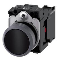
Pushbutton, 22 mm, round, plastic with metal front ring, black, pushbutton, flat, momentary contact type, with holder, 1 NC, screw terminal, with laser labeling, symbol number according to, ISO 7000 or IEC 60417
