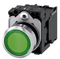
Illuminated pushbutton, 22 mm, round, metal, shiny, green, pushbutton, flat, momentary contact type, with holder, 1NO, LED module with integrated LED 110 V AC, screw terminal, with laser labeling, symbol number according to, ISO 7000 or IEC 60417
