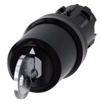
Key-operated switch IKON, 22 mm, round, plastic, special lock, with 2 keys, 3 switch positions I-O<II, left latching, right momentary contact type, actuating angle  $2x45^{\circ}$ , 10:30h/12h/13:30h, Key removal O+I
