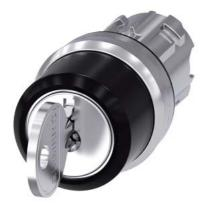
RONIS key-operated switch, 22 mm, round, metal, shiny, lock number SB30, with 2 keys, 3 switch positions I-O-II, latching, actuating angle 2x45°, 10:30h/12h/13:30h, Key removal I+O+II, possible special locks: SB31, 421, 455, Z=50-unit packaging
