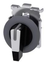
Selector switch, illuminable, 30 mm, round, Metal, matte, white, selector switch, long, front ring for flush installation, 3 switch positions I-O-II, latching, actuating angle 2x45°, 10:30h/12h/13:30h, with laser labeling, lower case
