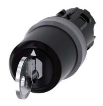
Key-operated switch IKON, 22 mm, round, plastic with metal front ring, lock number 360012K1, with 2 keys, 3 switch positions I-O<II, left latching, right momentary contact type, actuating angle 2x45°, 10:30h/12h/13:30h, key removal O+I, with laser labeling, lower case
