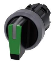
Selector switch, illuminable, 22 mm, round, plastic with metal front ring, green, selector switch, short, 3 switch positions I-O-II, latching, actuating angle  $2x45^{\circ}$ , 10:30h/12h/13:30h, Z=50-unit packaging
