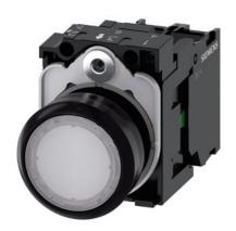
Illuminated pushbutton, 22 mm, round, plastic, white, pushbutton, flat, momentary contact type, with holder, 1NO, LED module with integrated LED 24 V AC/DC, screw terminal, with laser labeling, upper case
