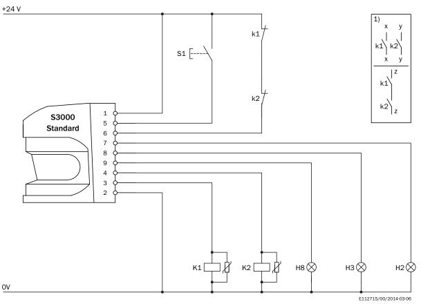
S3000 Standard in conjunction with relays/contactors
