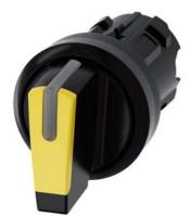
Selector switch, illuminable, 22 mm, round, plastic, yellow, selector switch, short, 3 switch positions I>O<II, momentary contact on the left, latching on the right, actuating angle  $2x45^{\circ}$ , 10:30h/12h/13:30h, with laser labeling, upper case and lower case, always upper case at the beginning of the word
