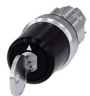
key-operated switch Siemens, 22 mm, round, metal, shiny, lock number SSG10, with 2 keys, 3 switch positions I-O-II, latching, actuating angle 2x45°, 10:30h/12h/13:30h, key removal I, with laser labeling, upper case and lower case, always upper case at beginning of line
