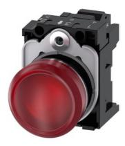
Indicator light, 22 mm, round, metal, shiny, red, lens, smooth, with holder, LED module with integrated LED 110 V AC, spring-type terminal, with laser labeling, upper case and lower case, always upper case at beginning of line
