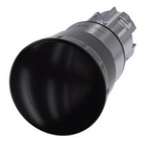
Mushroom pushbutton, 22 mm, round, metal, shiny, black, 40 mm, positive latching, acc. to EN ISO 13850, rotate-to-unlatch, with laser labeling, inscription or symbol Customer-specific selection with SIRIUS ACT configurator (CIN)
