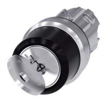
RONIS key-operated switch, 22 mm, round, metal, shiny, lock number SB30, with 2 keys, 2 switch positions O-I, latching, actuating angle 90°, 10:30h/13:30h, key removal O+I, possible special locks: SB31, 421, 455, Z=50-unit packaging
