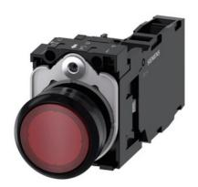
Illuminated pushbutton, 22 mm, round, plastic, red, pushbutton, flat, momentary contact type, with holder, 1 NO+1 NC, LED module with integrated LED 110 V AC, screw terminal, with laser labeling, upper case and lower case, always upper case at beginning of line
