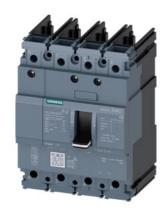
circuit breaker 3VA5 UL frame 125 breaking capacity class S 25kA @ 480V 4-pole, line protection TM210, FTFM, In=100A overload protection Ir=100A fixed short-circuit protection Ii=10 x In N conductor unprotected without connection
