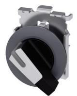
Selector switch, illuminable, 30 mm, round, Metal, matte, white, selector switch, long, front ring for flush installation, 2 switch positions O<I, momentary contact type, Actuating angle 45°, 10:30h/12h, with laser labeling, upper case
