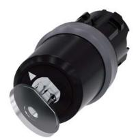
Key-operated switch BKS, 22 mm, round, plastic with metal front ring, lock No. E9 (VW), without key, 2 switch positions O-I, latching, actuating angle  $90^{\circ}$ , 10:30h/13:30h, key removal O+I, with laser labeling, upper case
