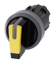
Selector switch, illuminable, 22 mm, round, plastic with metal front ring, yellow, selector switch, short, 3 switch positions I>O<II, momentary contact on the left, latching on the right, actuating angle 2x45°, 10:30h/12h/13:30h, with laser labeling, upper case
